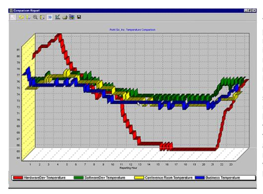
The dynamic HTML page displays on each row the following sensor information: name, serial number, age since last reception, service mode indicator, readings and units. All readings are shown in engineering units. The image to the left is a monitored temperature trend using the Pointware application software, measuring four temperatures over 24 hours.
